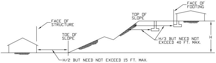
**R403.1.7 Footings on or adjacent to slopes.** The placement of buildings and structures on or adjacent to slopes steeper than 1 unit vertical in 3 units horizontal (33.3-percent slope) shall conform to Sections R403.1.7.1 through R403.1.7.4.
